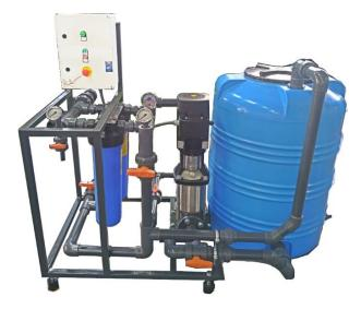
Clean in place procedure restores flux and rate of water purification of used reverse osmosis membranes. During operation, RO membranes are clogged with mineral (scaling), organic (fouling) and microbial (biofilm) deposits.
